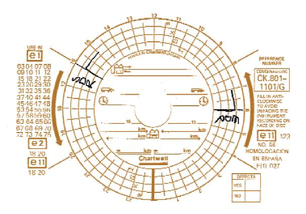
This is an example of manual entries made on the rear of a tachograph chart of a driver who started his day at 06.00 with an hour's work doing other duties away from his vehicle. He also finished his day with an hour of other work away from his vehicle and has indicated both the end and the start of a daily rest period. His activities while with the vehicle are recorded by the instrument on the other side of the chart once it has been inserted.
